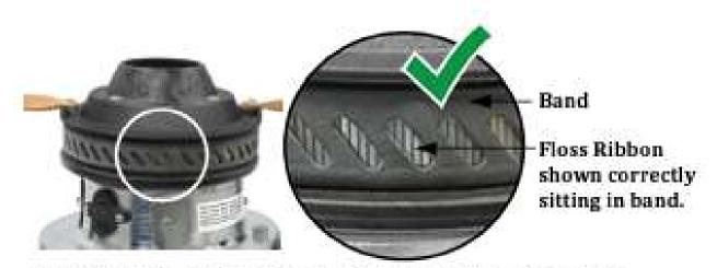
Step 4: Check the floss ribbon(s) (heating element) located inside the head assembly; make sure it has not shaken out of the band during transportation. If ribbon is out of band, push it back into place manually, before plugging in machine.
